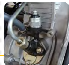
Direct injection Injection pump provides easy start and low fuel consumption
