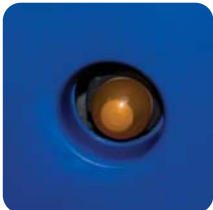
Fuel prime pump
